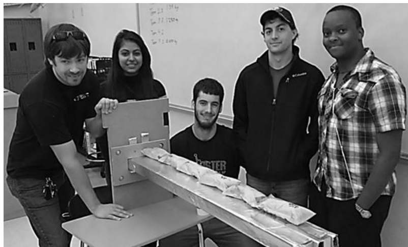
Figure 5. Test of multicell structure. Not only did it carry the specified loads but it also demonstrated a high level of rigidity.
