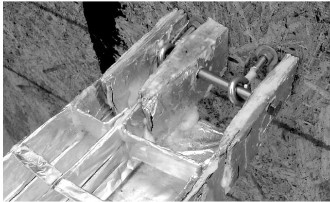
Figure 7. Detail of the root attachment of one of the concepts. Notice how the spars have been padded up for the bearing loads of the pin and on the wall.
