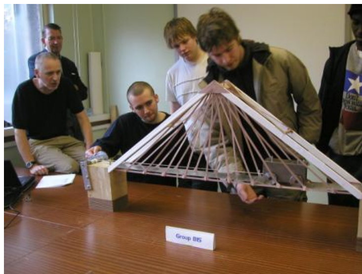
Figure 9. Unconventional truss geometry
