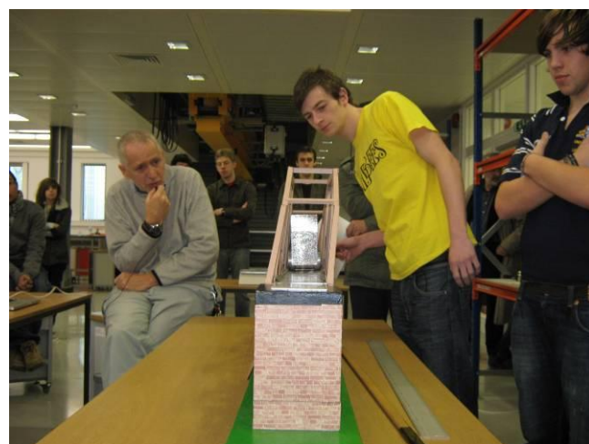
Figure 11. Lack of lateral stability during testing
