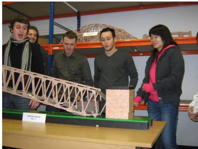
Figure 10. Two Week Creation – Part 2 – End connection failure
