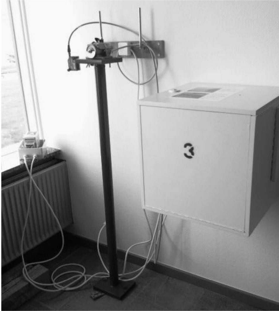
Figure 3. Test setup for the chimney. Displacements are measured with the laser fixed to the wall on the top.
