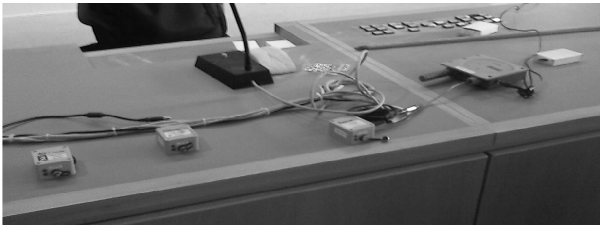
Figure 1. The sensors for CO 2 and temperature measurements placed on the teachers desk.
