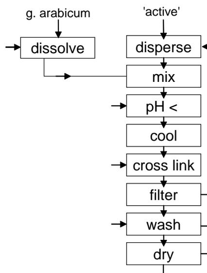
Figure 1. Flowsheet for production of polymer capsules containing a liquid herbicide
