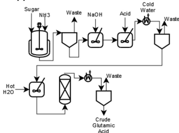
Figure 2. Process flowsheet for the production of glutamic acid.
