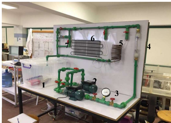
Figure 1. Plate (1) Designed and Built Hydraulic Bench including Pumps & Piping Systems 1-Water tank 2-Two identical pumps arrangements (can be operated as single, in series or in parallel) 3-Pressure gauge 4-Rotameter for flow measurements 5-Helical pipe 6-Tube banks 7-Gate valve and Globe valve
