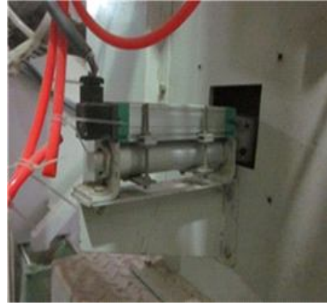
Fig. 3: Automatic device for measuring and monitoring the wear degree of two rubber shafts.
