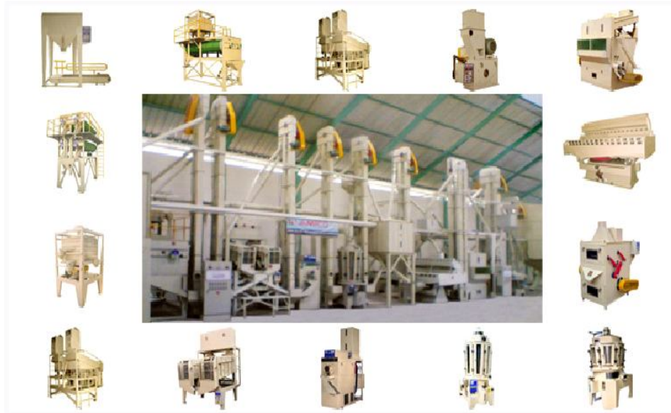
Fig.1: The rice milling line, made by Long An Manufacturing Company.
