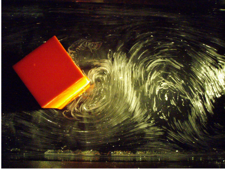
Figure 6. Vortices in the wake of a square cylinder visualised using glitter dust
