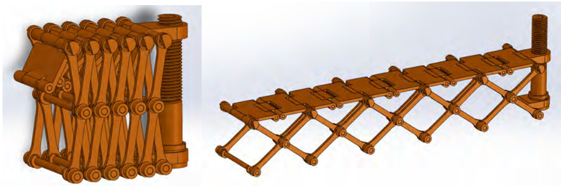
Figure 3: CAD of a bridge mechanism utilising a threaded power screw, scissor elements and tension locking top panels in (left) pre-deployment and (right) post-deployment.
