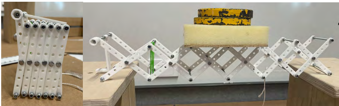
Figure 4: An elastic-powered bridge mechanism with hex-drive operated latch in its (left) pre-deployment and (right) post-deployment states.
