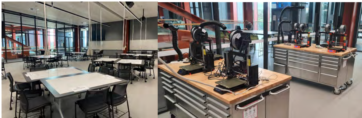
Figure 5: Our 120-seat, flat-floor teaching space (left). Two of our six mobile 3D printer workbenches, each featuring four Prusa i3 Mk3 printers and a ducted HEPA air filter (right).
