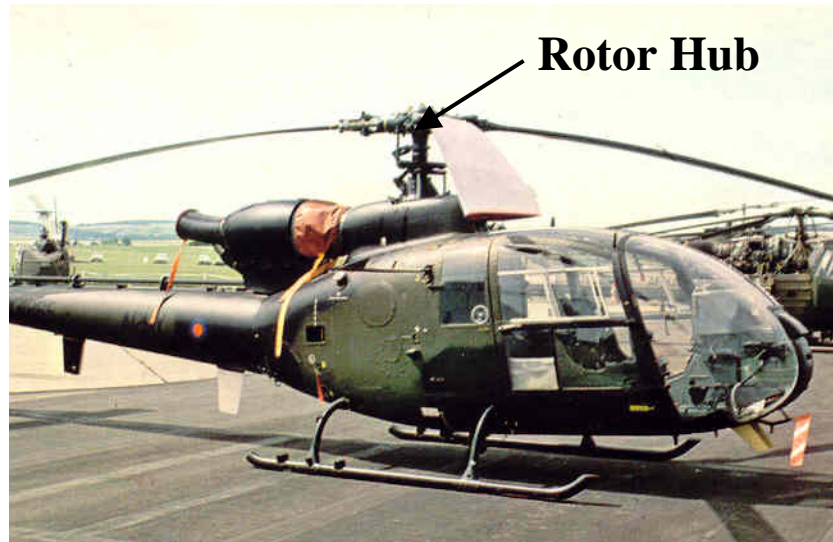
Figure 2 – An example of a helicopter rotor hub.
