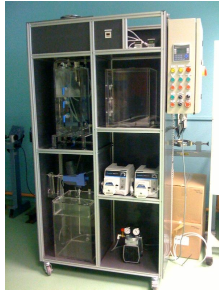
Figure 5. The Membrane Bio-reactor
