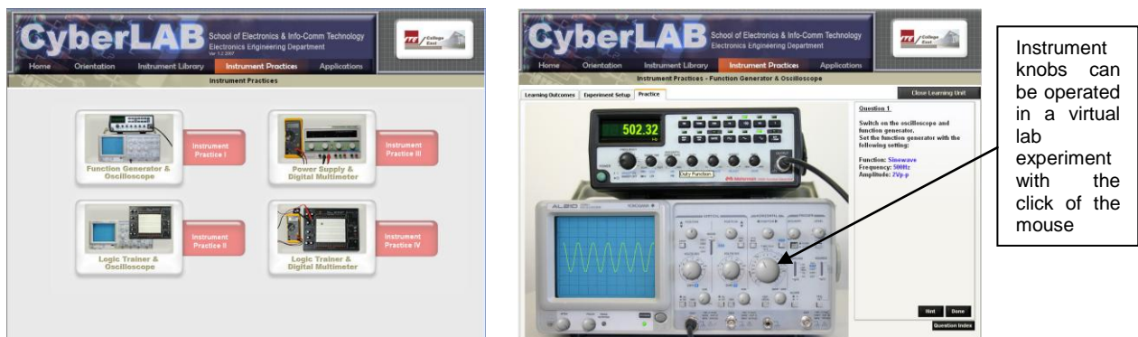
Figure 3. User Interface Design for ‘Instrument Practices’ - Function Generator & Oscilloscope
