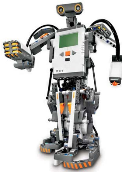
Figure 3. An example of a robot built using the Lego NXT platform [9].
