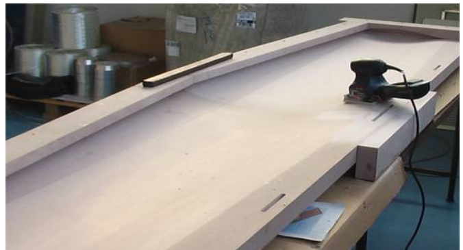
Fig. 10: CATIA solid model of the vertical/horizontal tail connection (left) and Stabilizer mould in preparation (right)
