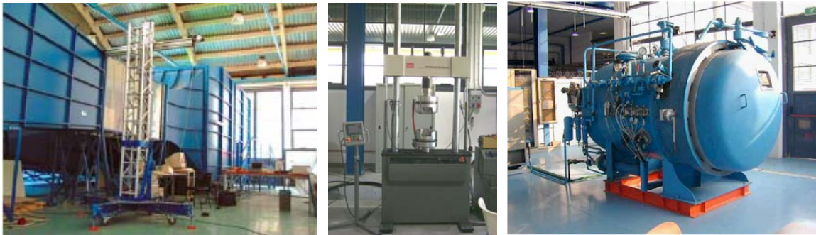
Figure 4: Low speed wind tunnel, MTS mechanical testing machine and autoclave.
