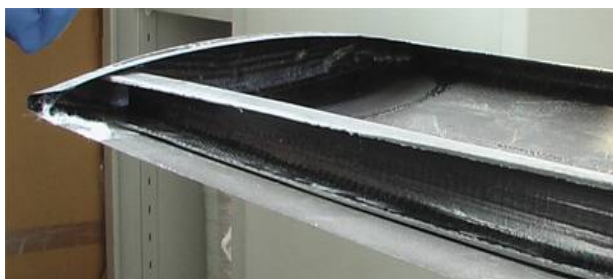
Fig. 11: Stabilizer tip detail before skin assembly (left) and a participant with his “creature” (right)
