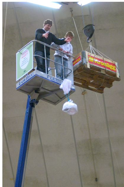
Figure 1. Assisting undergraduate students in the sky lift have just released a competing device, its parachute unfolding. Visible to the right is a crate suspended from a crane, by which the devices are elevated from ground level to the start position.
