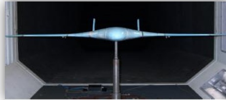
Figure 3. Half-scale model installed in the 7 by 5 ft wind tunnel in Sydney
