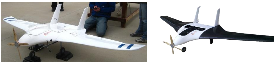
Figure 3. Hyperion 1.0 Flying Wing and Hyperion 2.0 Blended Wing Body (from left to right)
